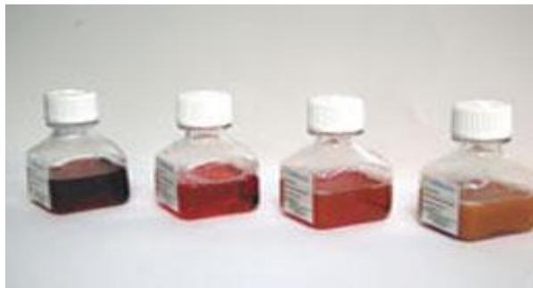
**Fig 3: Colours of various sized gold nanoparticles** (Source: [www.sigmaaldrich.com](http://www.sigmaaldrich.com))
