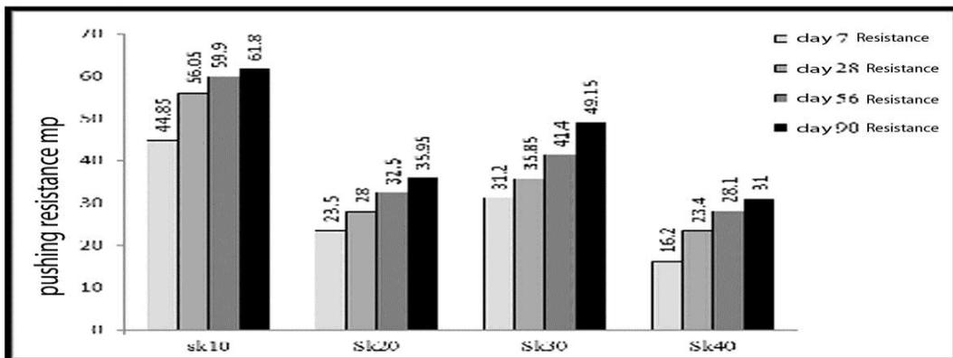
Figure 1 - compressive strength in the first phase
