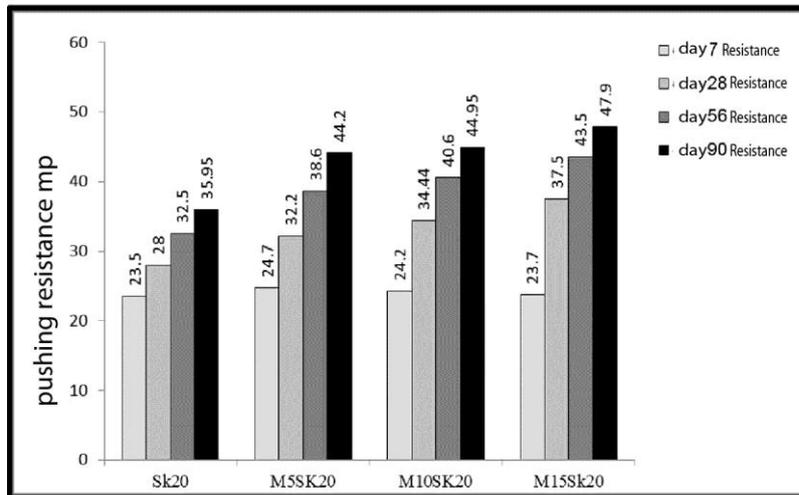
Figure 3 - compressive strength in the second phase
