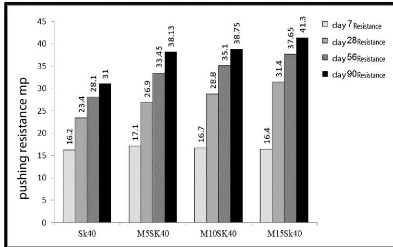
Figure 5 - compressive strength in the second phase
