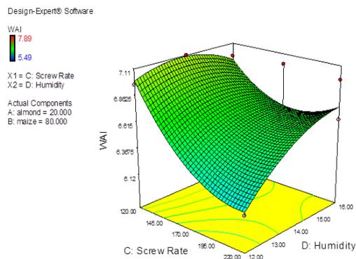
**Figure 1: Effect of humidity and the screw rate on the water absorption index**
