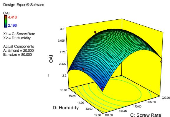
**Figure.3: Effect of humidity level and the screw rate on the oil absorbing index**
