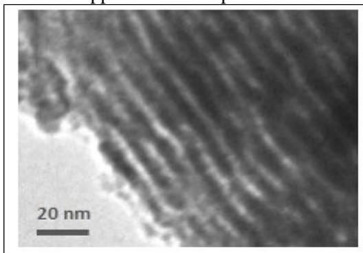
**Figure 1- Microscope Photo of Transmission electron microscopy (TEM) of CuO nanoparticles**
