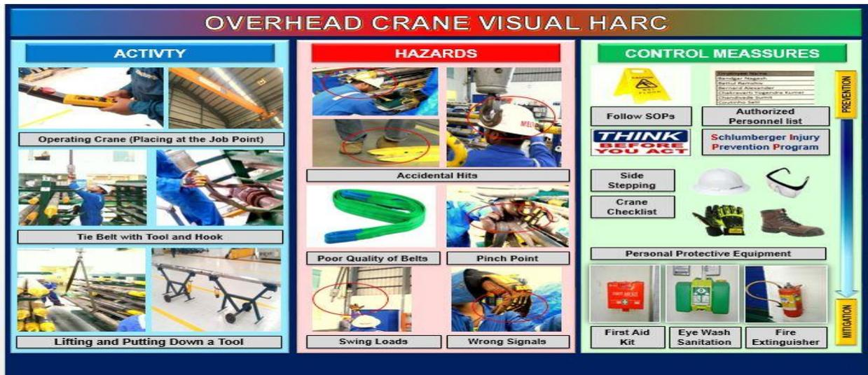
**Fig. 1 A typical Pictorial HIRAC for Overhead Crane Operation in Mumbai Base**
